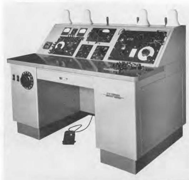
Figure 1. View of the console for preliminary electrical tests. The Type 716-C Capacitance Bridge is at the right, the Type 1231-B Amplifier and Null Detector at the top center of the pouch. At the left part face of the console is the Variac ® Autotransformer.
