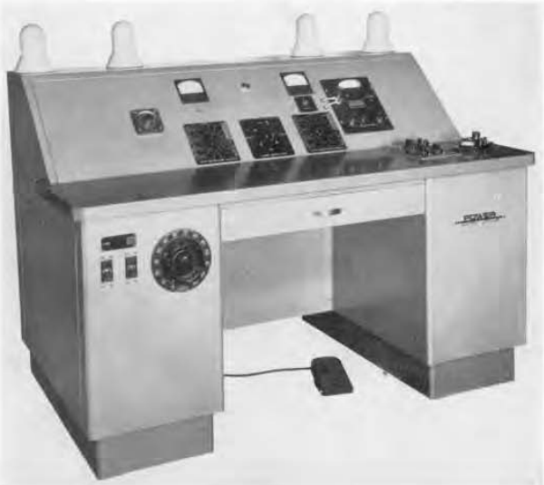
Figure 2. View of the console for final electrical tests. The General Radio Megohmmeter is at the right of the panel, and the Variac at the front face of the left-hand pedestal.
